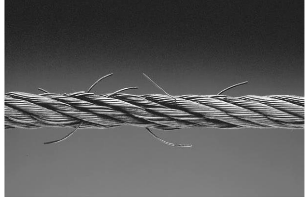
Cable With Broken Wires
